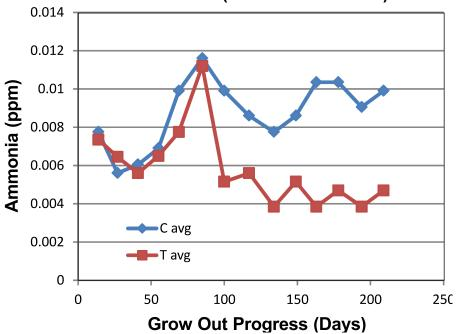
For the first 100 days (no StartSmart dosing), the test and control ponds showed identical ammonia concentration. Once StartSmart dosing began with the aerated mixing drum (14 day holding time), the ammonia reduction in the treated ponds was dramatic.
