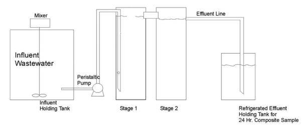
The dimensions of each of the main tanks (Stage 1 and Stage 2) was 1 and  $\frac{1}{2}$  feet square by 4 feet tall, with a total working volume of about 40 gallons each
