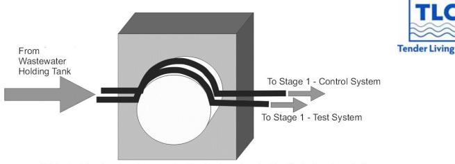
(Note dual feed system for ensuring identical wastewater feed to test and control)
