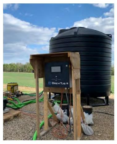
Based on the size of our farm we decided to set up a custom BrewTus to best meet our needs. This included a BrewTus 1000, a 5000 gallon tank for brewing and a 5000 gallon tank for storing brewed ACF SR. We purchased an additional aeration assembly for the storage tank just incase the ACF needed to be fed again.
