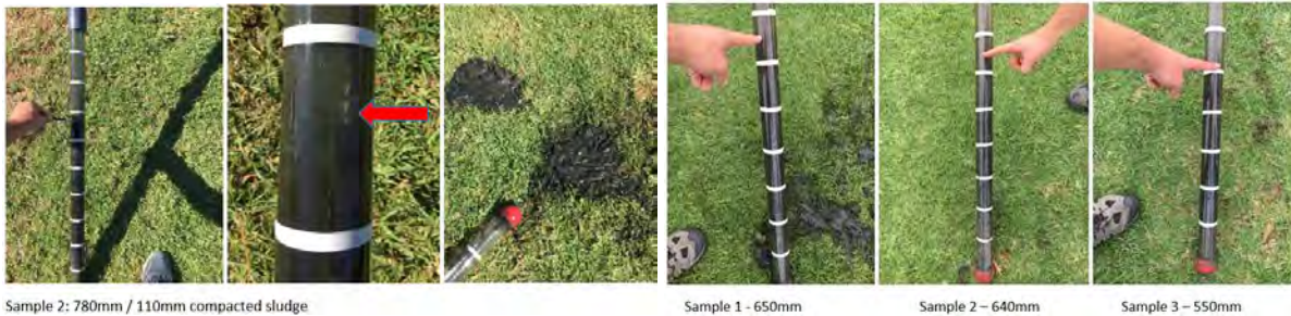
Sample 2: 780mm / 110mm compacted sludge
