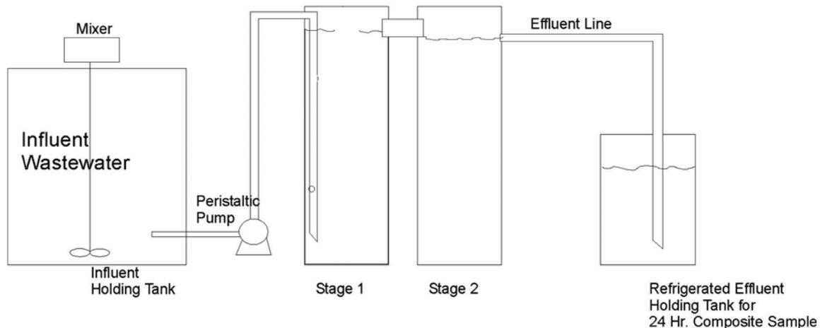
The dimensions of each of the main tanks (Stage 1 and Stage 2) was 1 and ½ feet square by 4 feet tall, with a total working volume of about 40 gallons each
