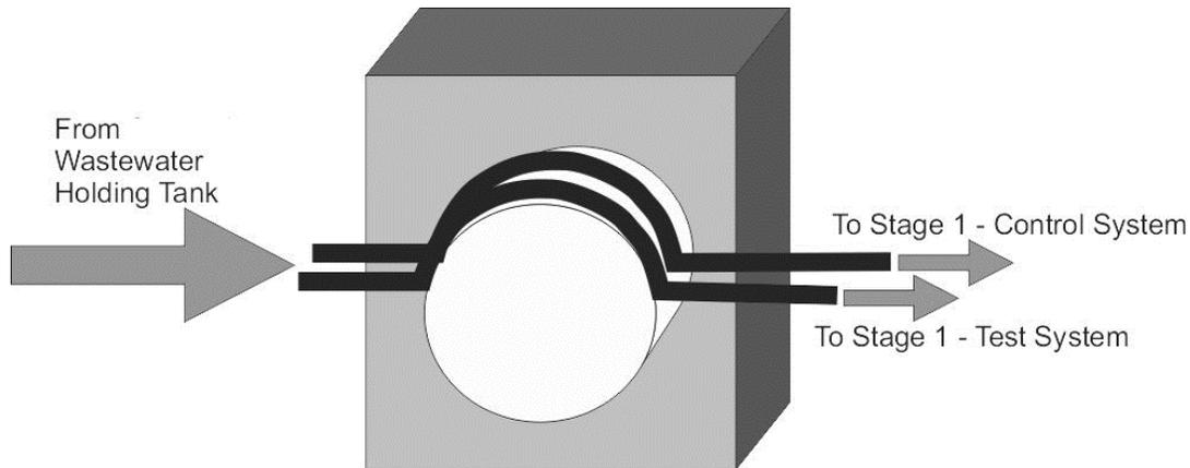
*(Note dual feed system for ensuring identical wastewater feed to test and control)*
